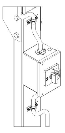
This TPI disconnect kit is intended for use with TPI High Velocity Fans mounted to TPI Floor Stands. It may be used without Floor Stand accessories but additional mounting hardware may be required.
