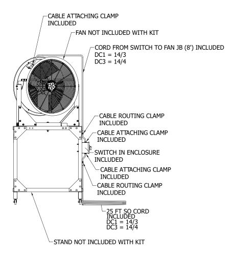
Choose mounting location for switch. Holes are precut on either side of the Floor Stands: one on the vertical tubing, and one on the horizontal tubing. Use supplied bolts and nylon insert nuts to secure to frame.
